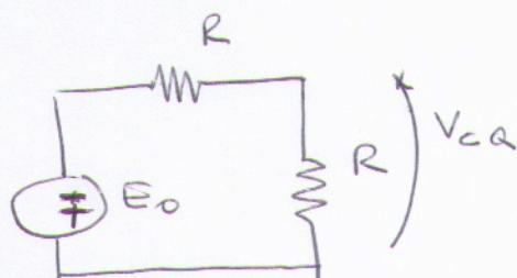
$$\boxed{V_{CQ} = -\frac{E_o}{2} = -8 \text{ V}}$$
