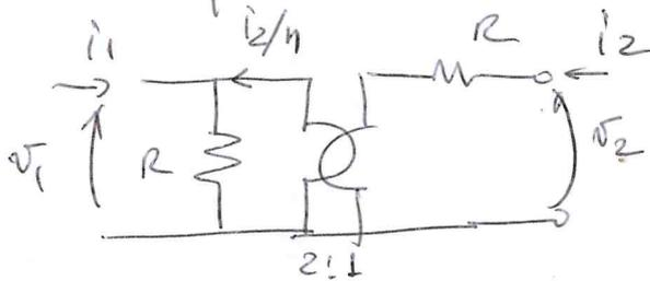
$$v_1 = R \left( i_1 + \frac{i_2}{n} \right)$$
