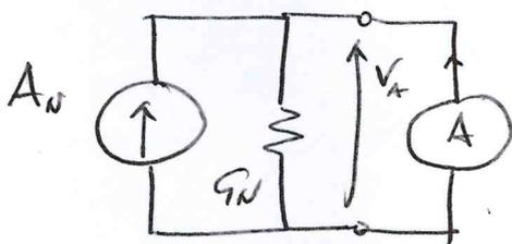
$$V_A = \frac{A_N + A}{G_N} = 25 \text{ V} \quad (15 \text{ V})$$
