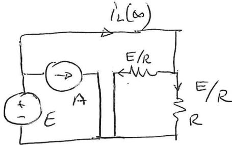
$$\tau = \frac{L}{R_{\text{eq}}}; \quad R_{\text{eq}} = \frac{R}{2} = 1\text{k}\Omega$$
